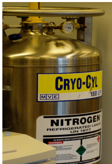
Figure 9: A tank of liquid nitrogen, used to supply a cryogenic freezer (for storing laboratory samples at a temperature of about -150 °C)
